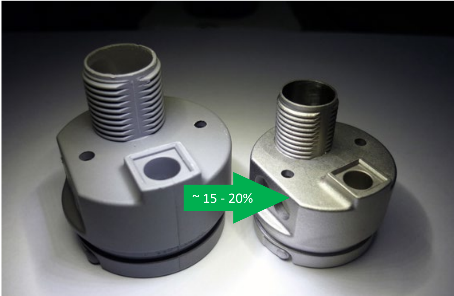
Metal Injection Molded housing cover made from 316L stainless steel (sensor casing). Before and after sintering. (source PIM International Vol.4 No.1, March 2010)
